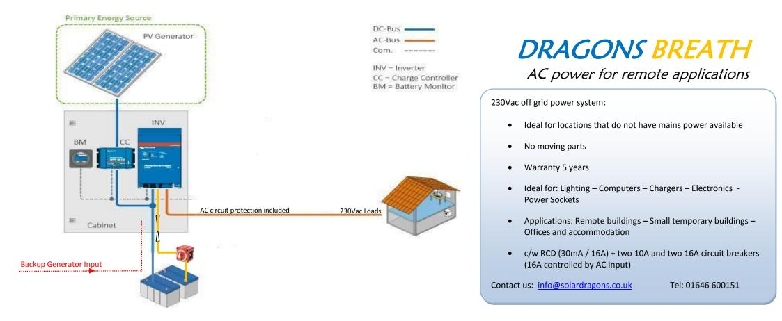
Self contained 230vac 50hz power solution combines MPPT solar panel charge controller, with inverter/charger and AC circuit distribution in one unit.
